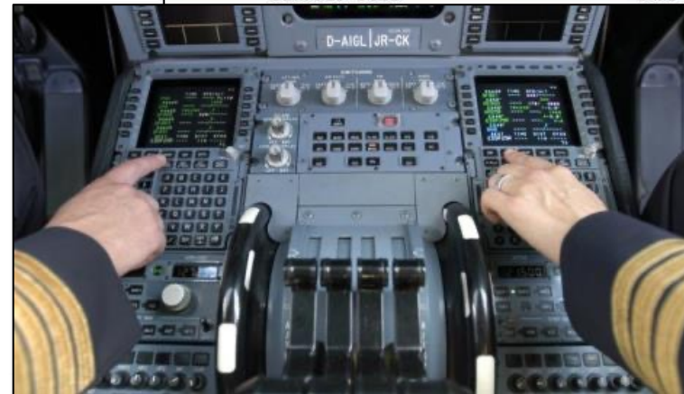
Crew entry of the flight plan
