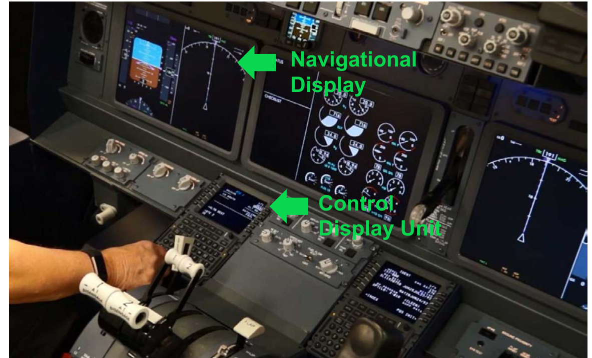
Cockpit interfaces to the FMS
