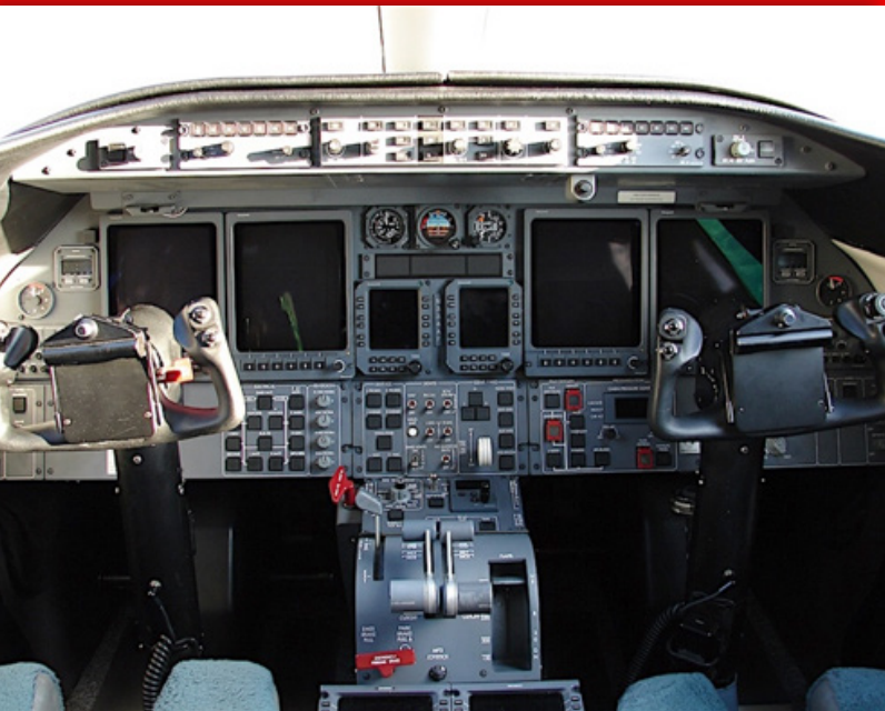
The Old: The original CRT-based Learjet 45 cockpit.
