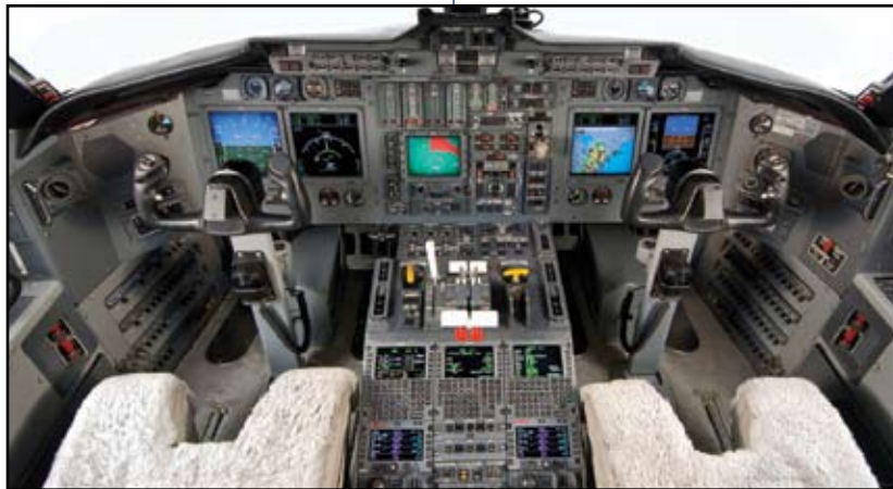
Duncan Aviation’s Glass Box Project solution for the Challenger 600/601-1A, Universal’s EFI 890R.
