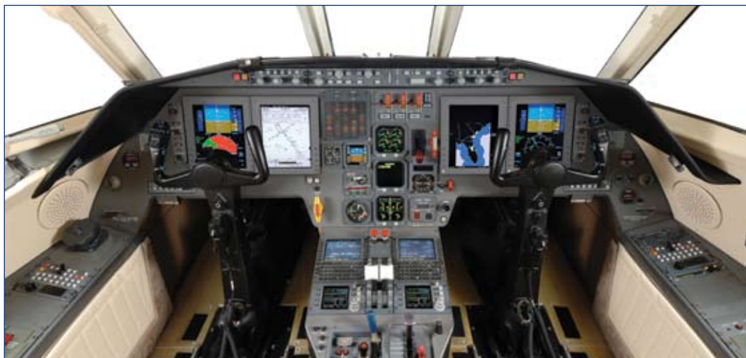
Duncan Aviation's conceptual Glass Box Project solution for the Falcon 2000. The first installation is scheduled for late summer 2008.
